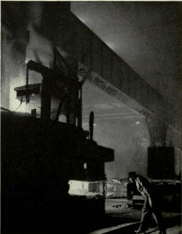
Another quality control—samples of steel are frequently taken from the electric furnace for analysis.
